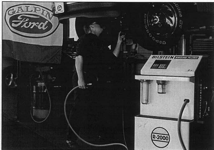
The Bilstein R-2000 Engine Flush System circulates a detergent through an engine's oil passages and lubricated internals to clean out the built-up sludge and other contaminants that remain in the engine even after an oil change.
